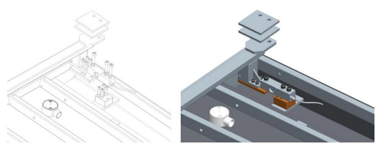
NOTE: use cable ties through existing holes under the steelwork to attach cable and junction box assembly.
